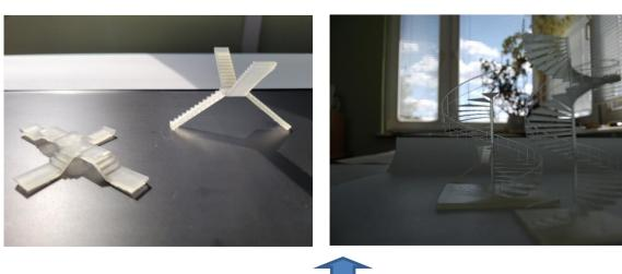
The 3D printed (in SLA) models of roof fragments and stairs
