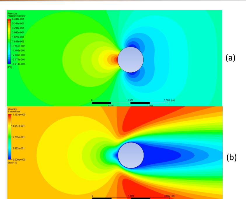
Figure 1. Pressure (a), velocity (b) contours for cylinder, for Re=10000
