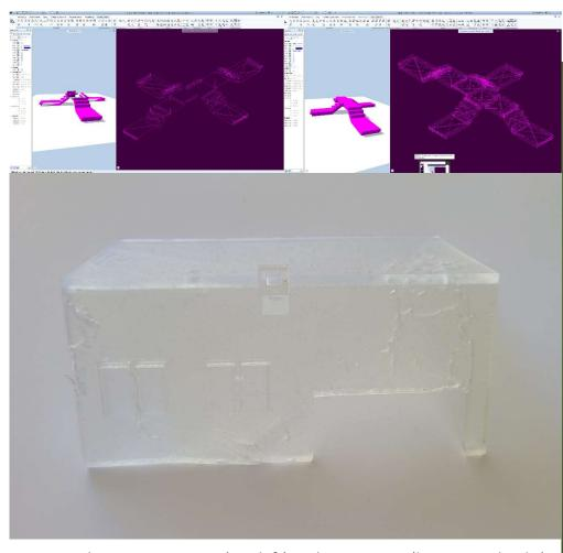
Errors during preparation (top left) and 3D printing (bottom and right)
