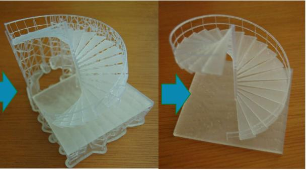
A few basic steps of preparing a 3D print of spiral staircase (design in computer application, adding supports and setting orientation, raw print and ready model)
