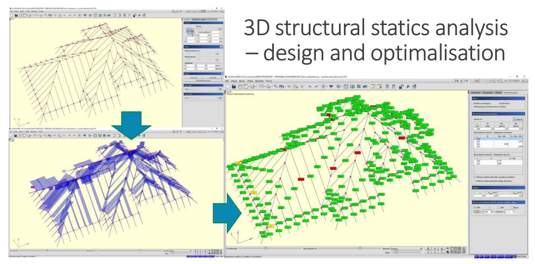
Example of structural statics analysis in Rama 3D, the program of ArcadiaSoft (geometry, load and stress of structure cross-sections)
